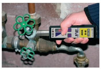
For starting a measurement the Aqua M-40 device is beeing attached with the accessories found in the scope of delivery to any available spot on the pipeline or valves. If the pipe has a leakage the leak noise will be audible on this spot as well. The integrated LED display is indicating the intensity of the heard leakage born noise.
