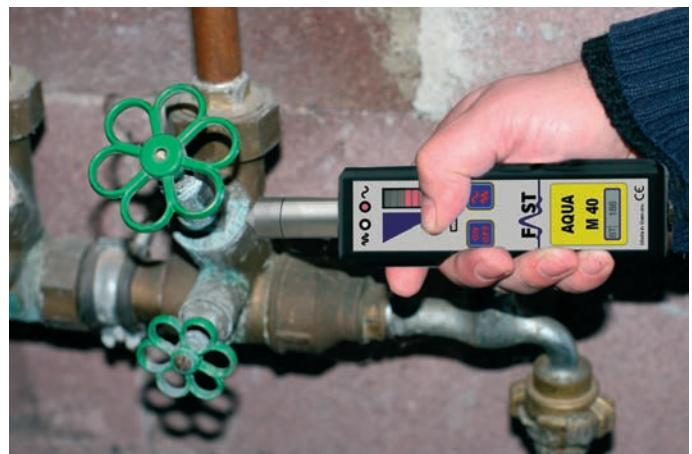
For starting a measurement the Aqua M-40 device is being attached with the accessories found in the scope of delivery to any available spot on the pipeline or valves. If the pipe has a leakage the leak noise will be audible on this spot as well. The integrated LED display is indicating the intensity of the heard leakage born noise.
